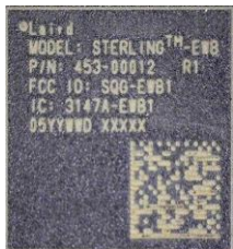
Figure 1 Sterling-EWB Base SiP module (453-00012)
