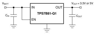
Figure 8-7. TPS7B81-Q1 Typical Application Schematic
