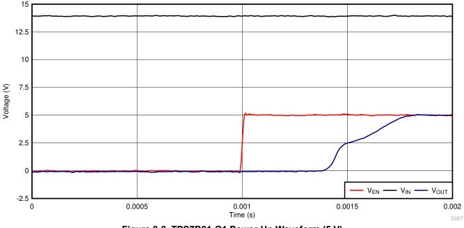
Figure 8-8. TPS7B81-Q1 Power-Up Waveform (5 V)
