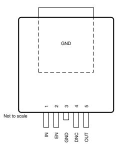
Figure 5-3. KVU Package, 5-Pin TO-252, Top View
