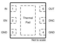
Figure 5-2. DRV Package, 6-Pin WSON PowerPAD<sup>™</sup>, Top View
