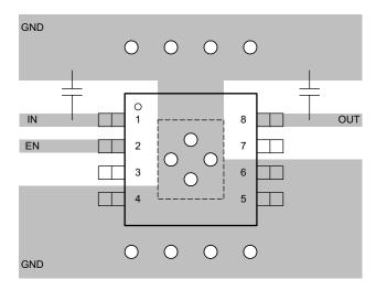
Figure 10-1. TPSB81-Q1 Example Layout Diagram
